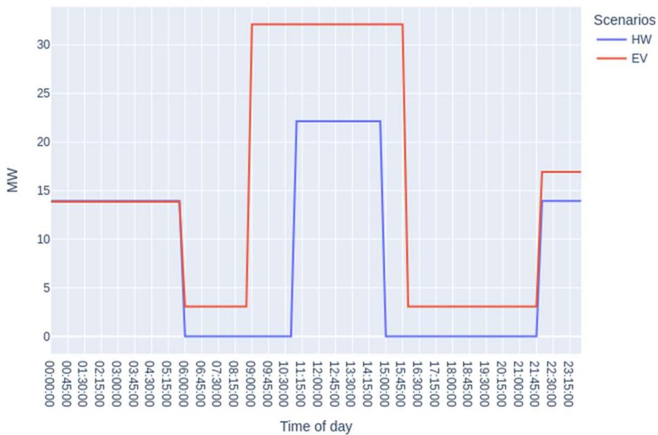
Figure 2. Second step in the method: shaped EV and water heating load profiles
