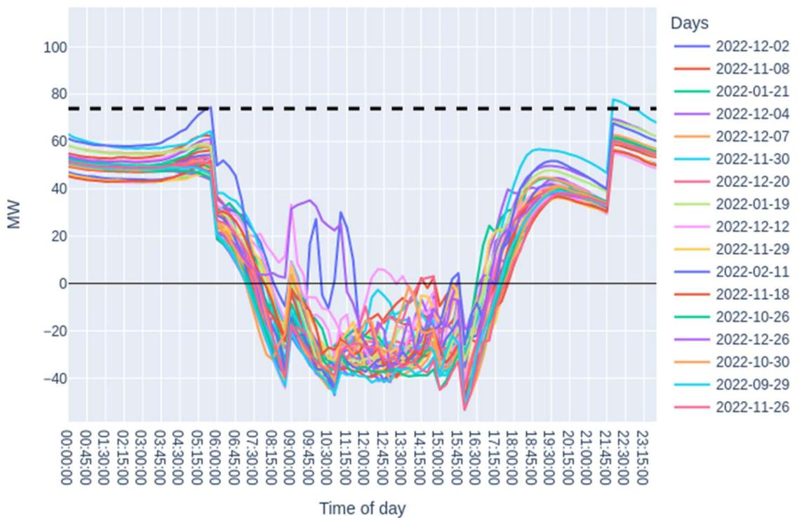
Figure 16. Substation loading on minimum demand days for High solar, High home EV scenario.
