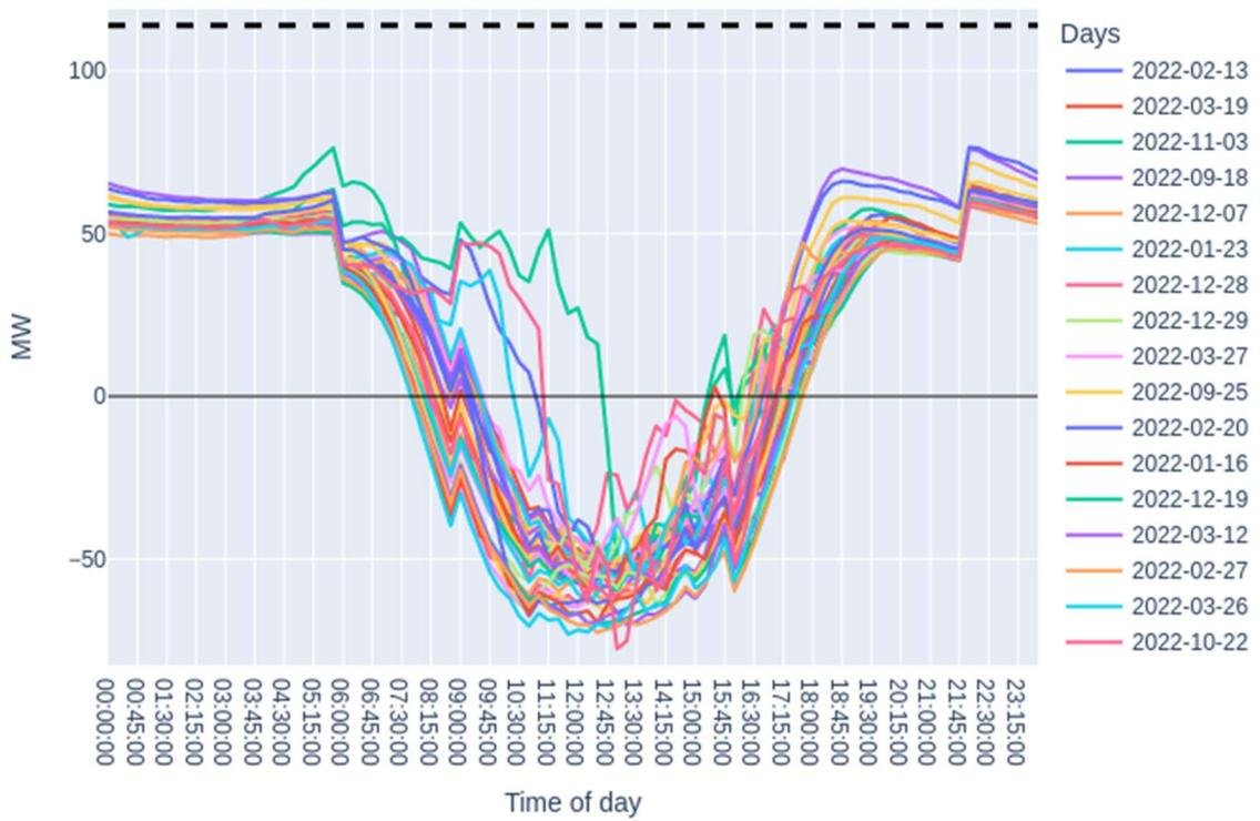
Figure 27. Substation loading on minimum demand days for High solar, High home EV scenario.
