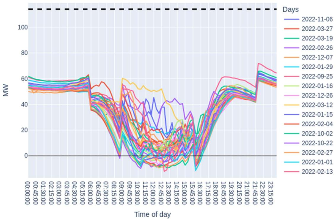
Figure 25. Substation loading on minimum demand days for Low solar, High home EV scenario.
