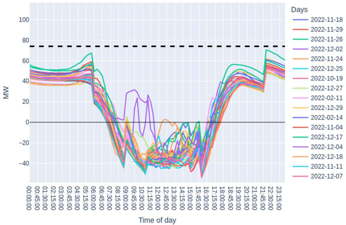
Figure 15. Substation loading on minimum demand days for High solar, Low home EV scenario.
