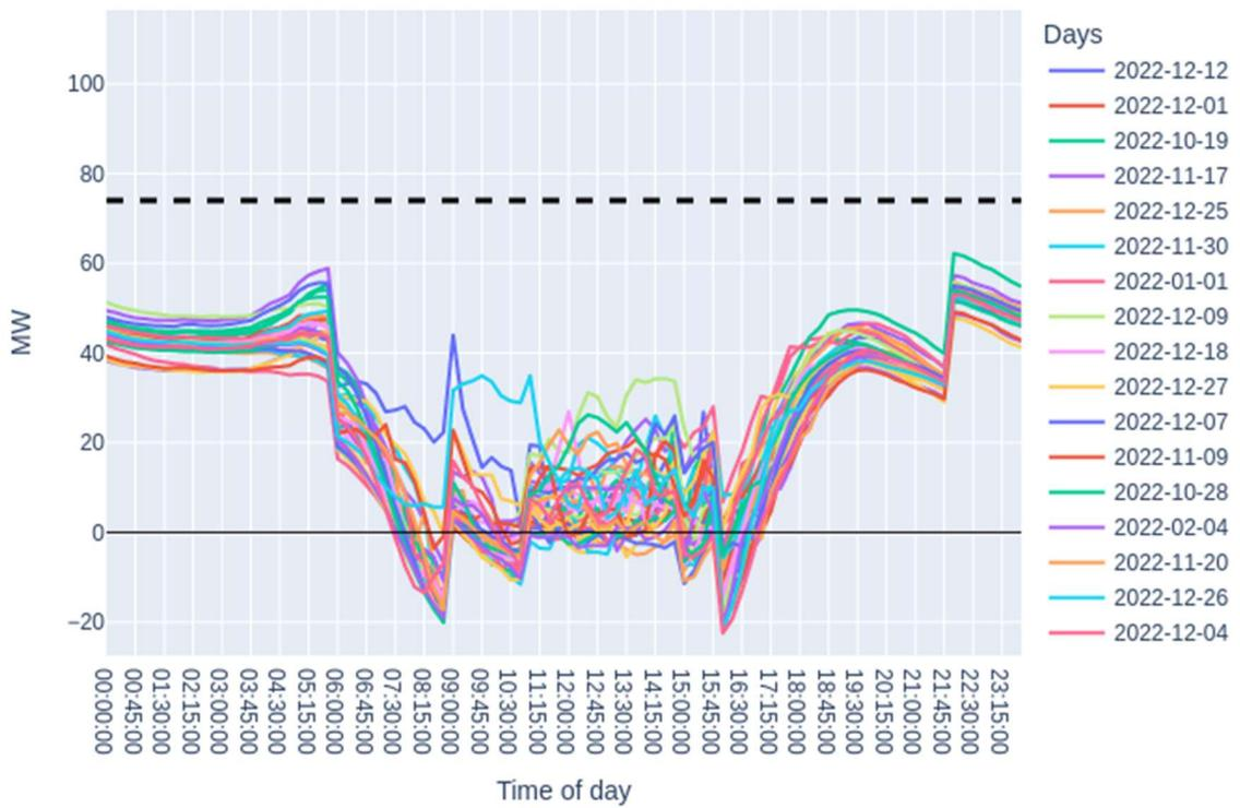
Figure 13. Substation loading on minimum demand days for Low solar, Low home EV scenario.
