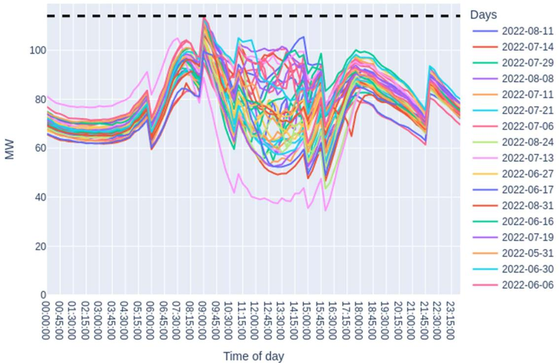
Figure 21. Substation loading on peak demand days for Low solar, High home EV scenario.
