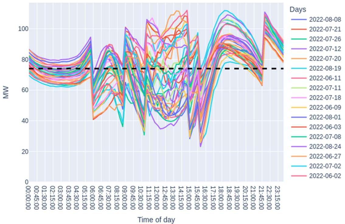
Figure 10. Substation loading on peak demand days for Low solar, High home EV scenario.
