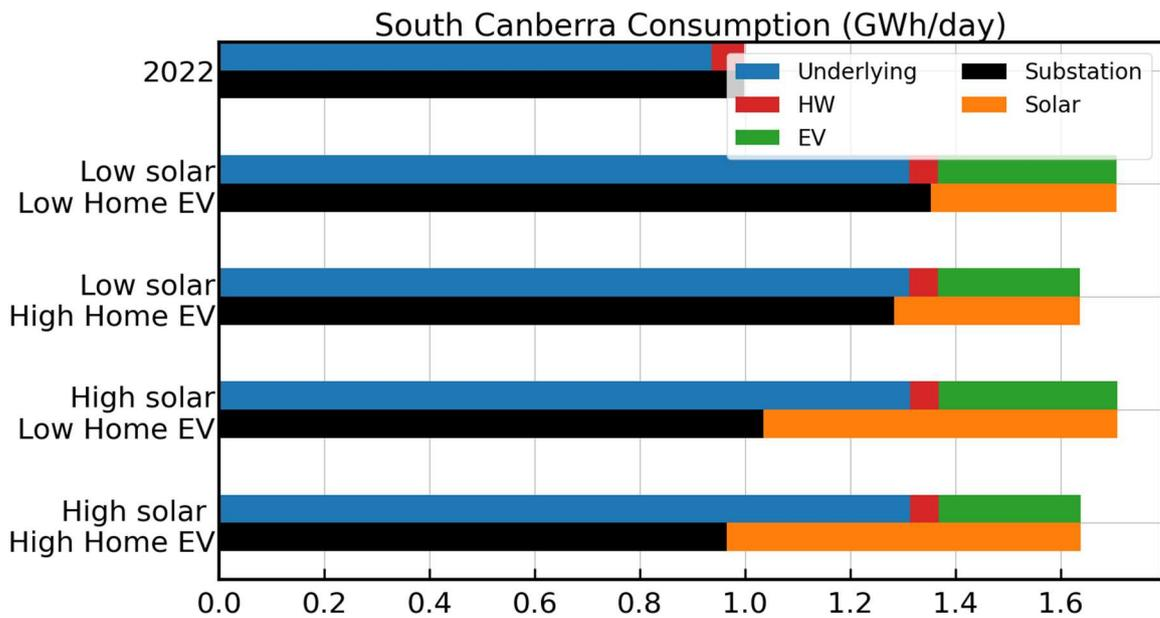
Figure 17. Electricity consumption in South Canberra in 2022 and in 2045 under 4 scenarios.
