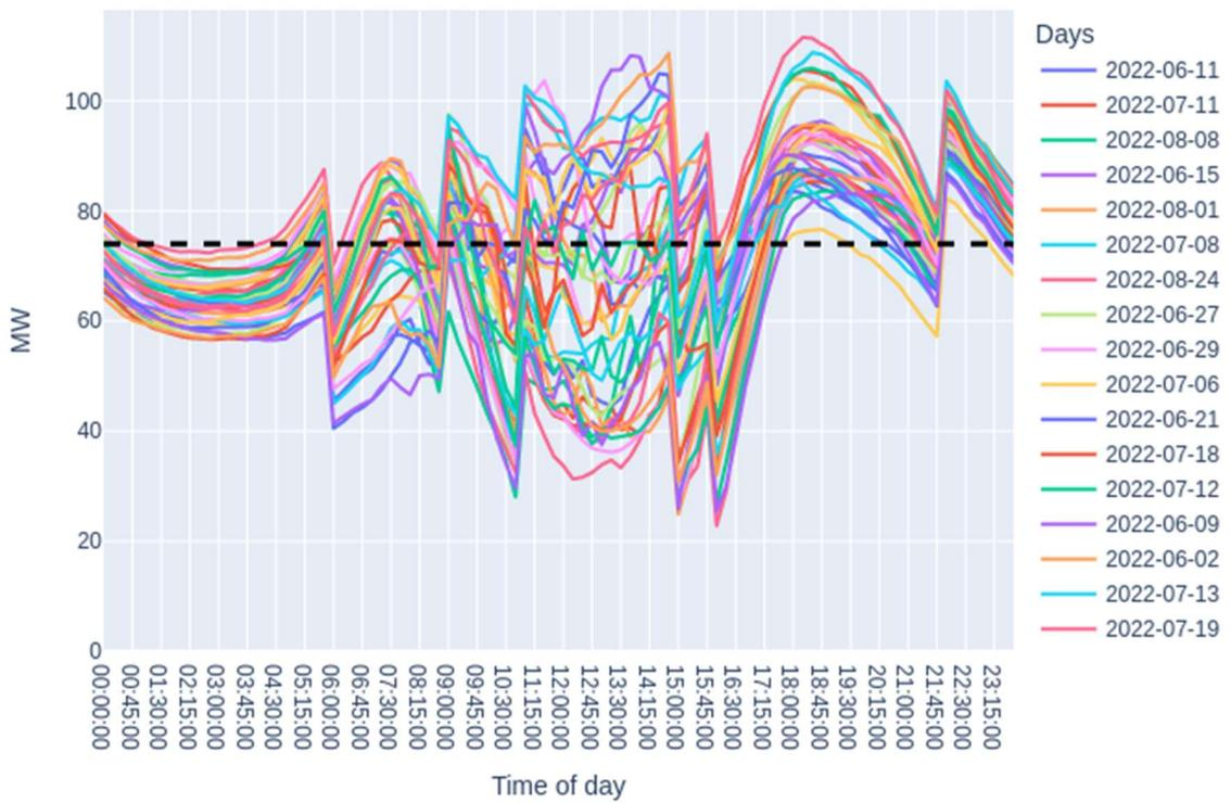
Figure 9. Substation loading on peak demand days for Low solar, Low home EV scenario.
