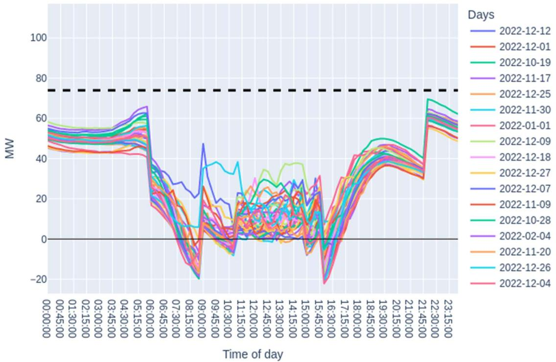
Figure 14. Substation loading on minimum demand days for Low solar, High home EV scenario.
