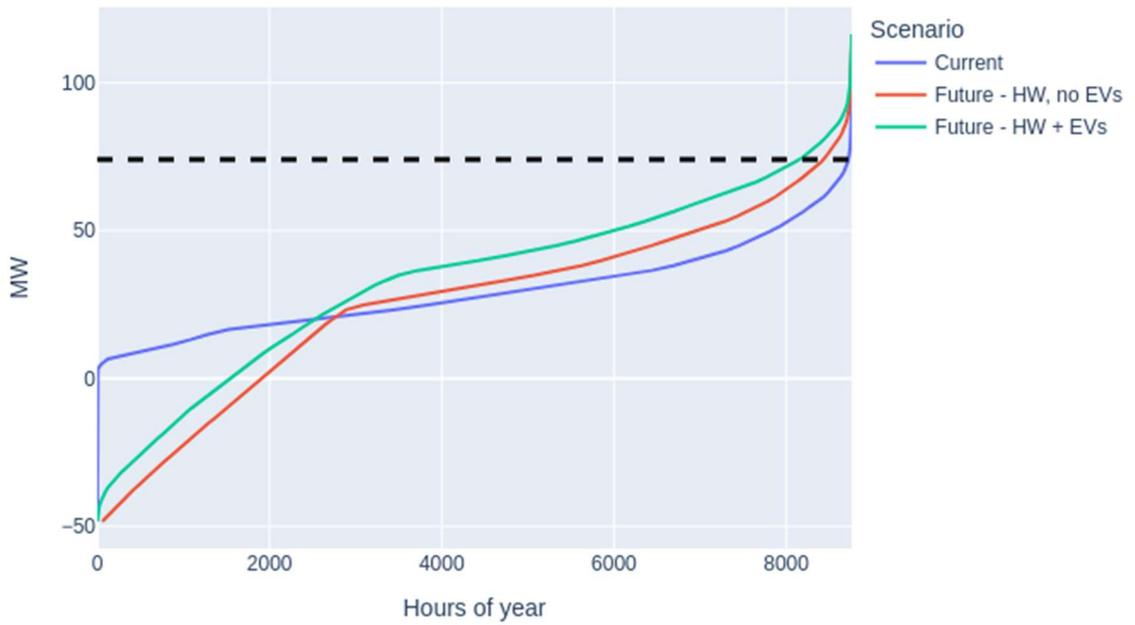
Figure 7. Load duration curve of Gungahlin substation loading under the High rooftop solar and Low home EV scenario, comparing distributions to current loading and loading without EVs.
