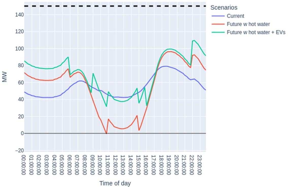
Figure 3. Final step in the method: adding EV and water heating loads to underlying demand
