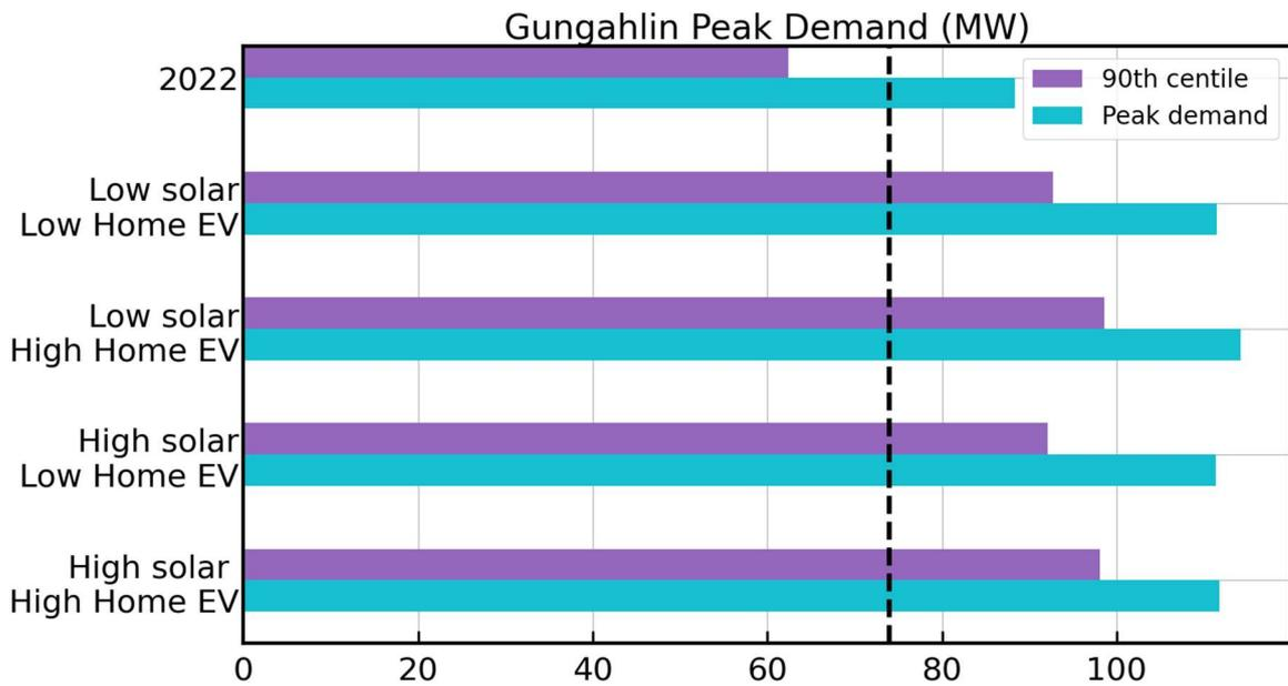
Figure 5. Peak demand and 90th centile in Gungahlin in 2022 and in 2045 under 4 scenarios. Dotted line indicates the current substation capacity.
