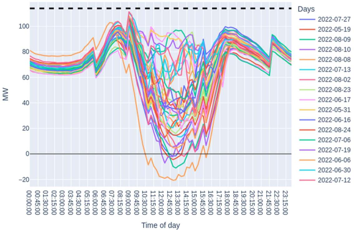
Figure 23. Substation loading on peak demand days for High solar, High home EV scenario.
