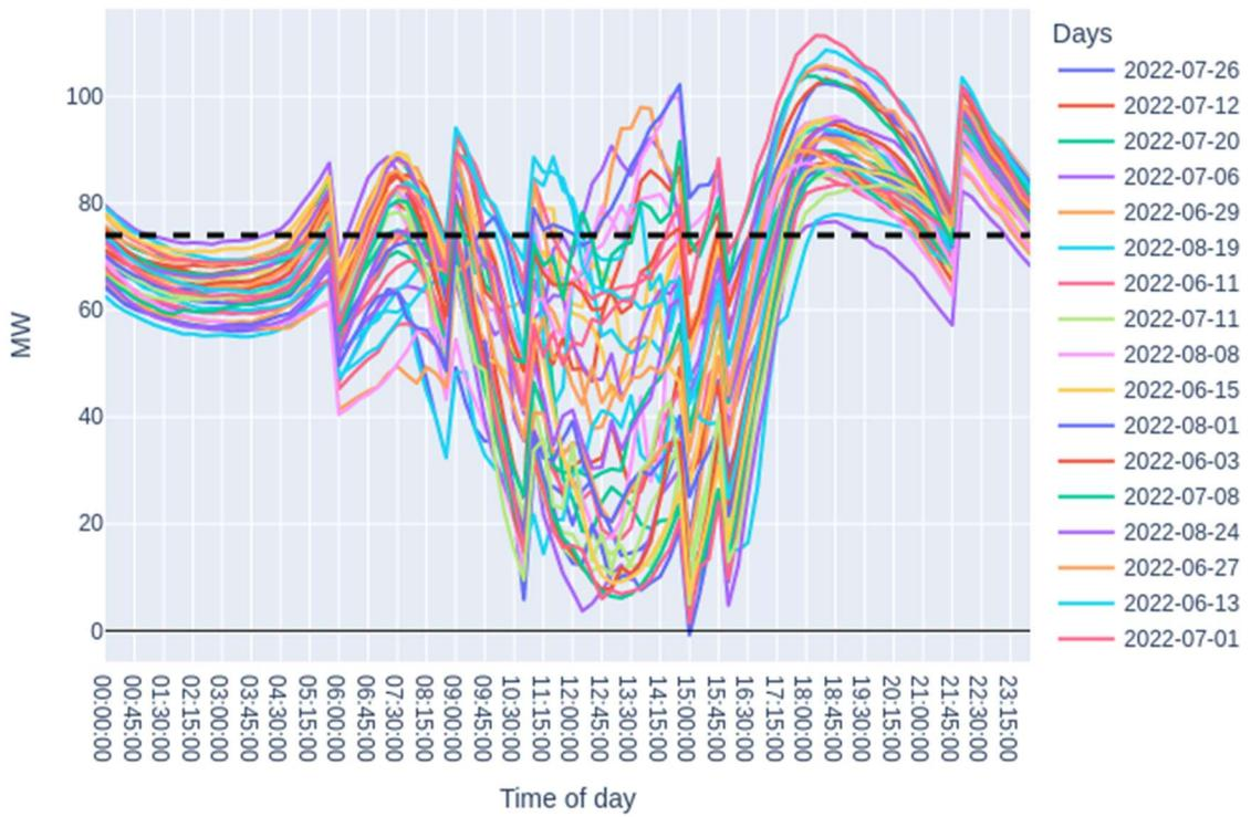
Figure 11. Substation loading on peak demand days for High solar, Low home EV scenario.
