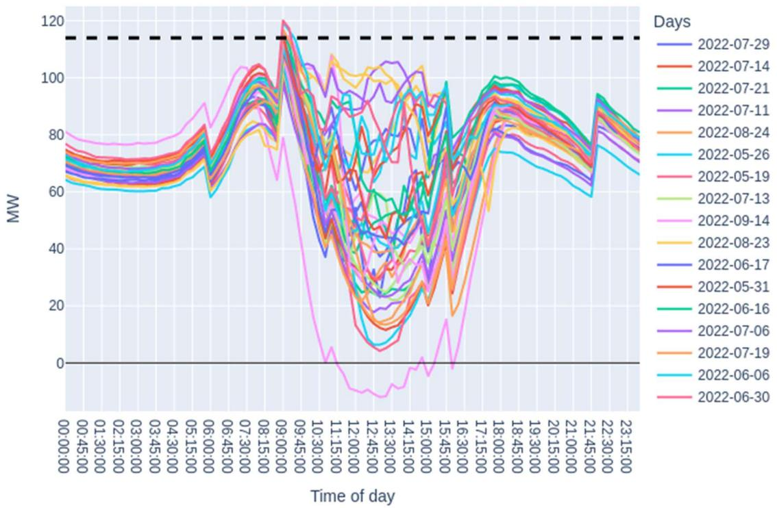
Figure 22. Substation loading on peak demand days for High solar, Low home EV scenario.
