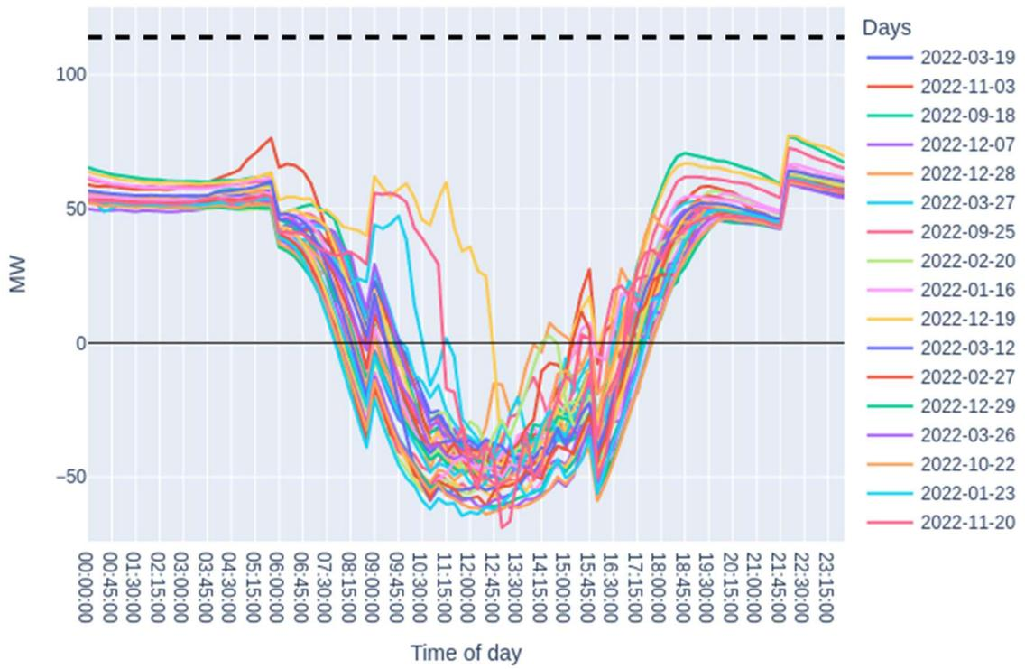
Figure 26. Substation loading on minimum demand days for High solar, Low home EV scenario.
