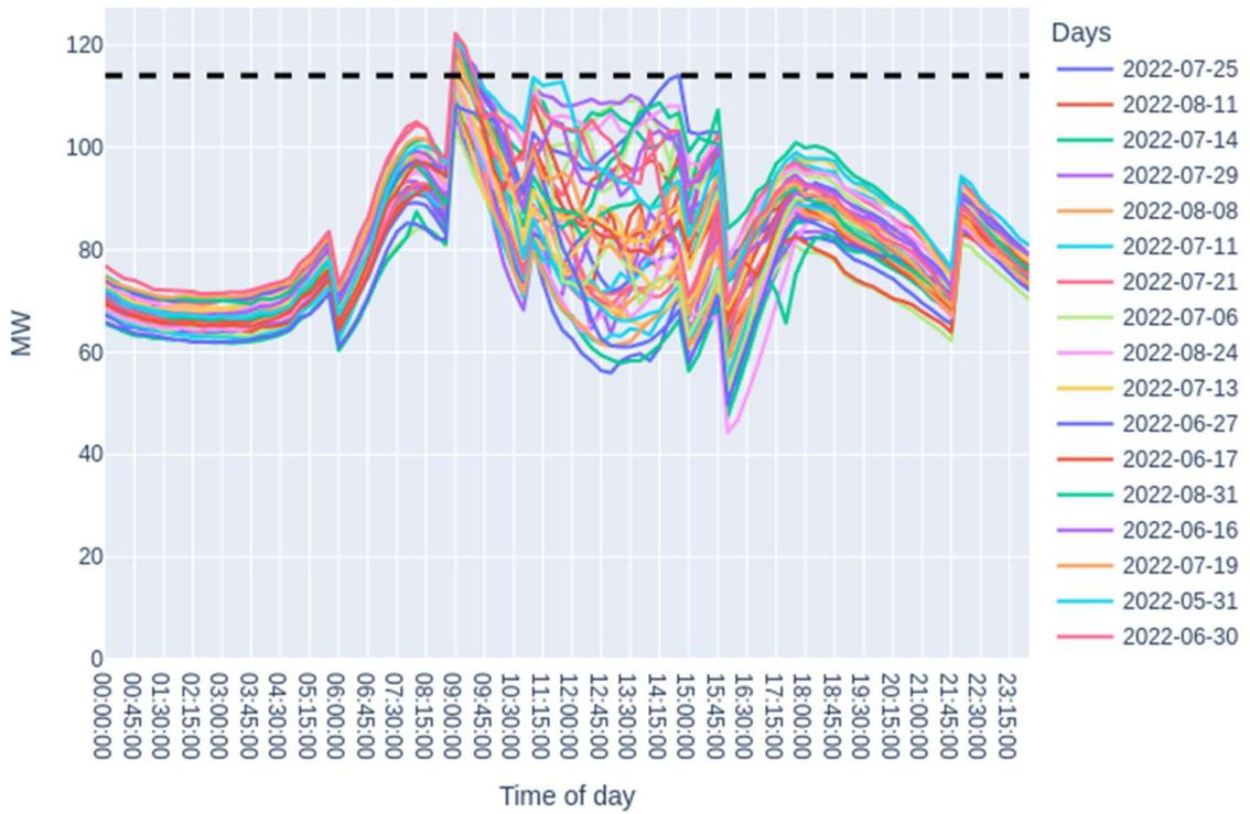
Figure 20. Substation loading on peak demand days for Low solar, Low home EV scenario.
