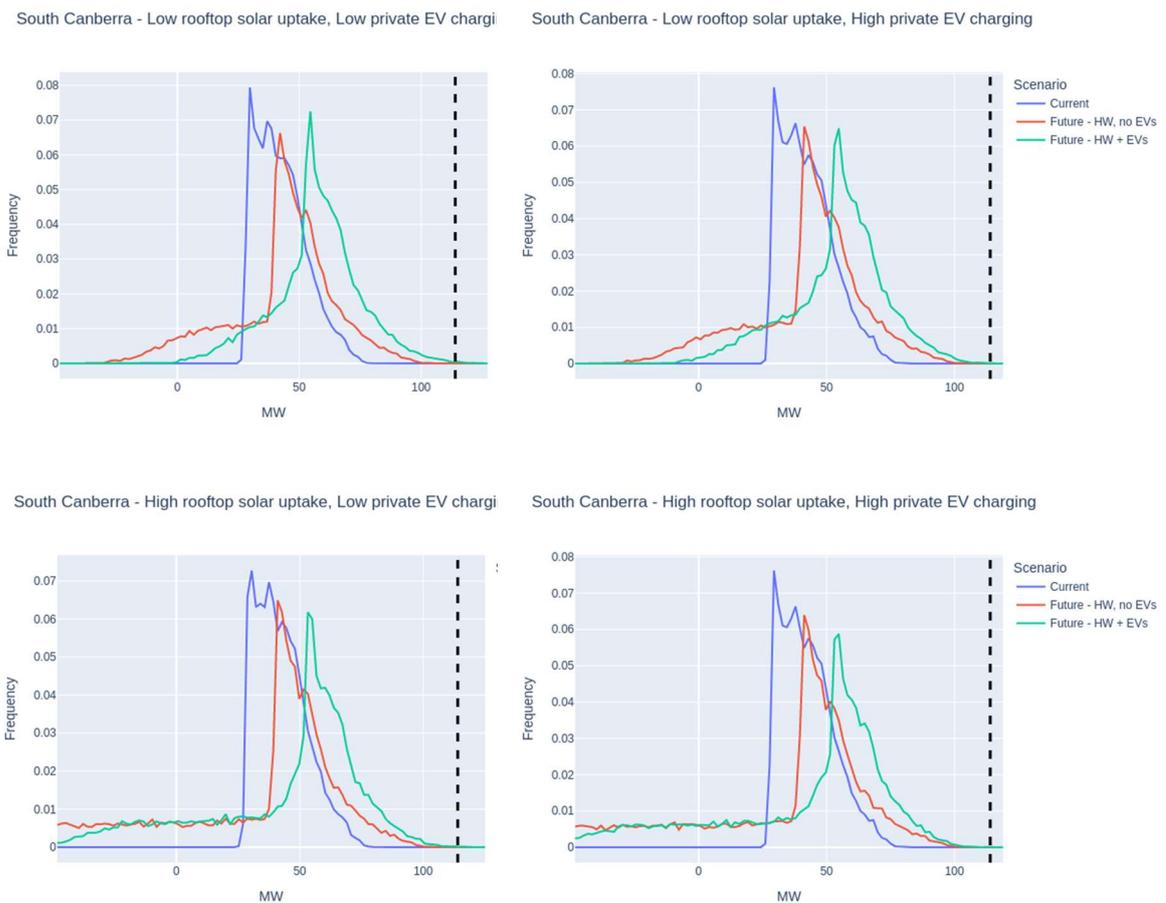
Figure 19. Frequency distributions of South Canberra substation loading under 4 scenarios, comparing distributions to current loading and loading without EVs.
