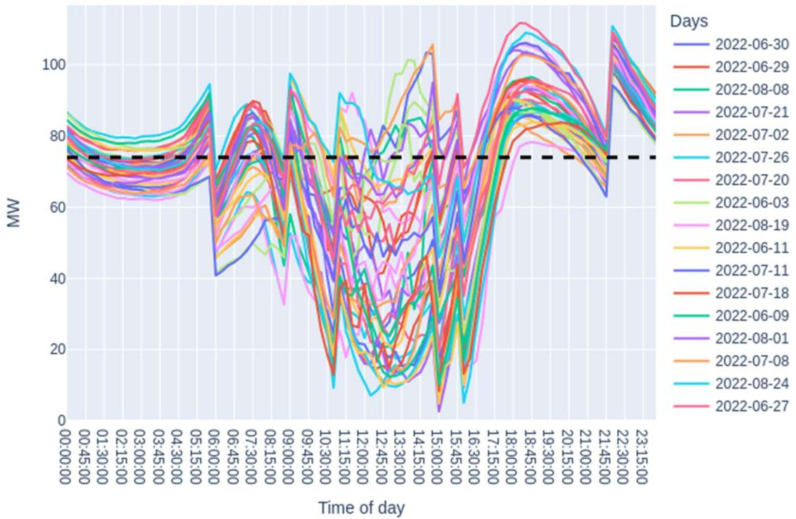
Figure 12. Substation loading on peak demand days for High solar, High home EV scenario.
