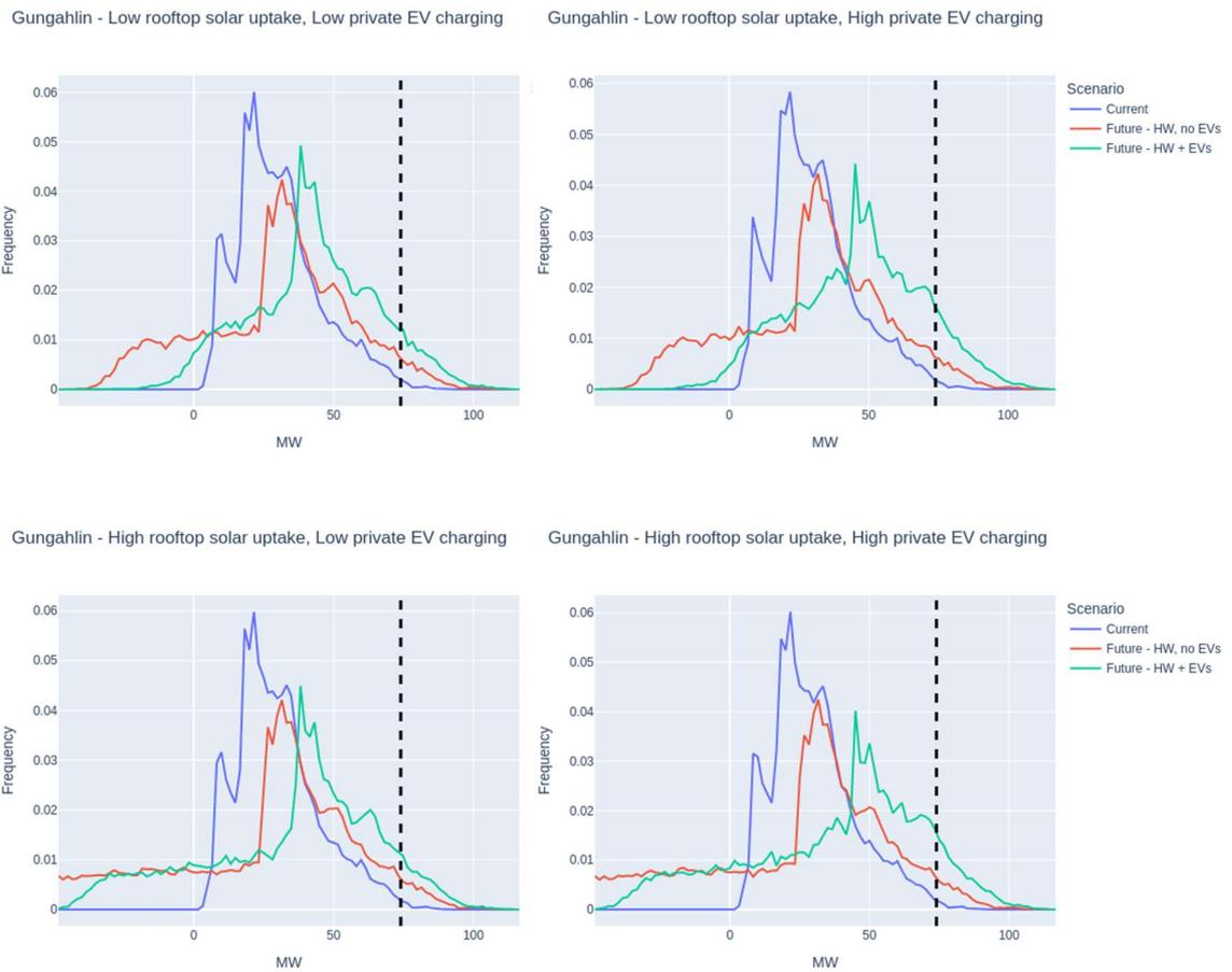
Figure 8. Frequency distributions of Gungahlin substation loading under 4 scenarios, comparing distributions to current loading and loading without EVs.
