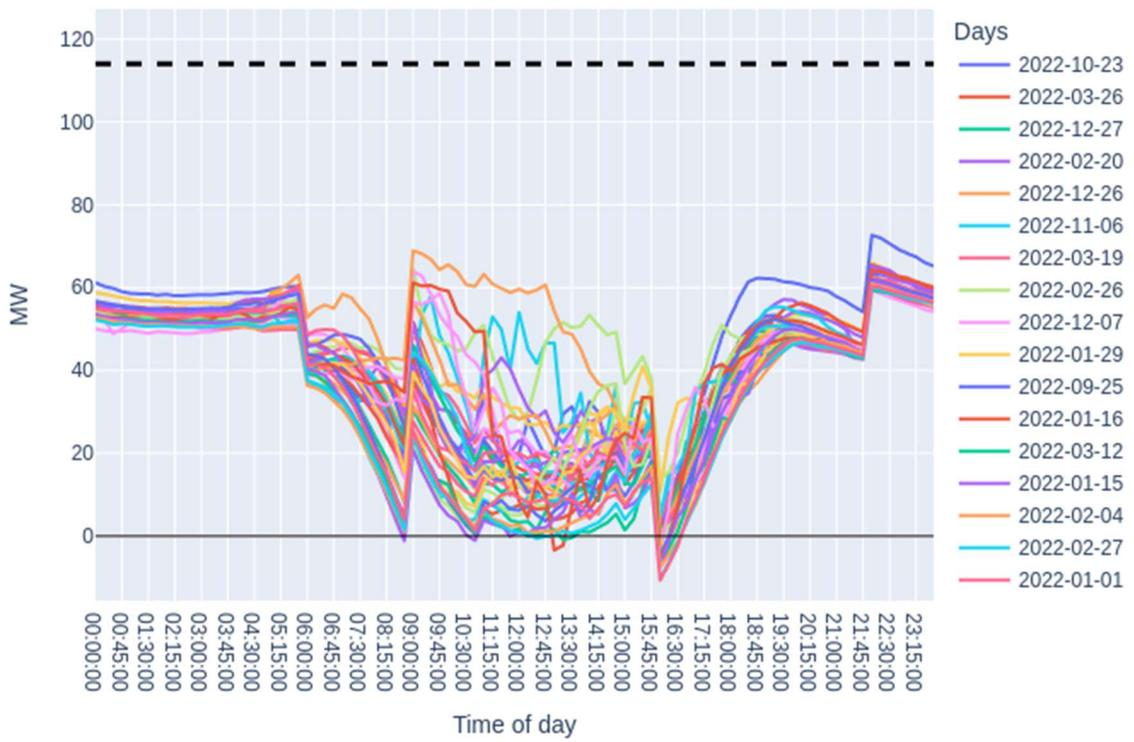
Figure 24. Substation loading on minimum demand days for Low solar, Low home EV scenario.
