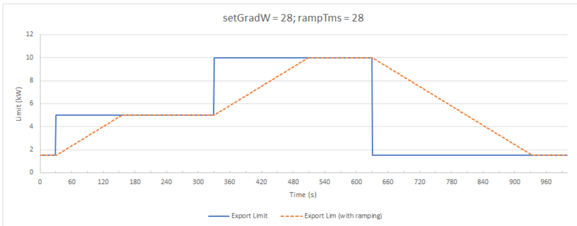
Figure 4: Example where rampTms and setGradW are the same.
