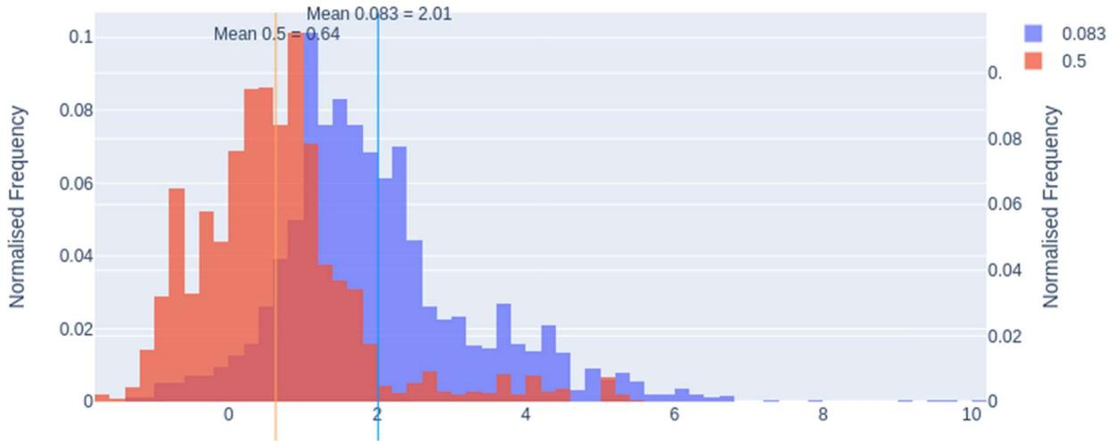
Figure 20 Distribution of zone substation loads during charging interval for low flexibility (*plug-in-fraction* of 8.3%, blue) and high flexibility (*plug-in-fraction* of 50%, red)
