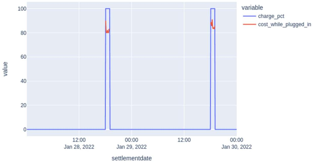
Figure 17 Best case charging scenario where EV is plugged in throughout the whole two-day period of 28<sup>th</sup> and 29<sup>th</sup> of January 2022. The EV can therefore charge at the absolute lowest cost moments - EV charging profile (in % of charger power capacity) shown in blue
