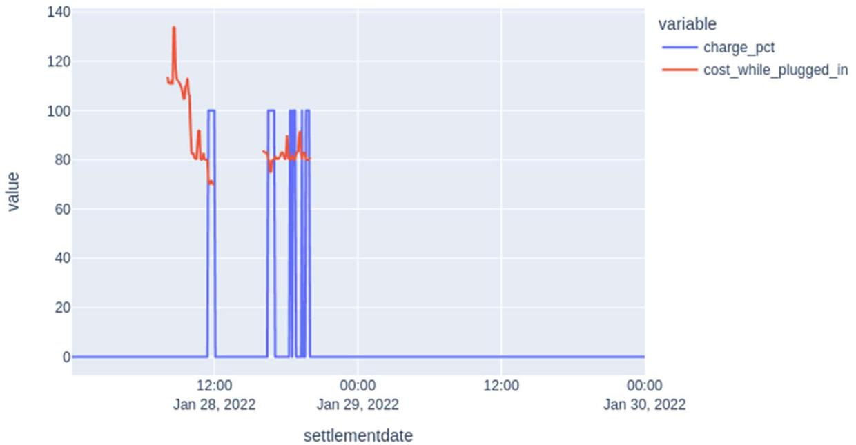
Figure 15 NEM price (red) during a 66% *plug-in-fraction plug-in-profile* on the 28<sup>th</sup> and 29<sup>th</sup> of January 2022. Also shown is the optimised EV charging profile (blue in % of charger power capacity), which selects the lowest cost times during this *plug-in-profile*
