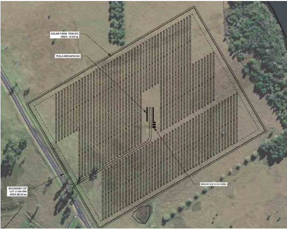
Figure 16 Illustrative design of a 4.99 MW solar farm on the outskirts of the community of Turros Heads
